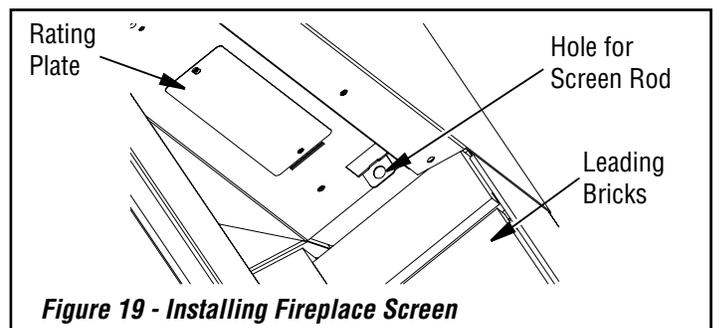
**Figure 19 - Installing Fireplace Screen**
