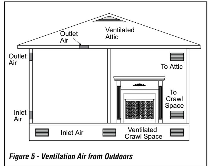
**Figure 5 - Ventilation Air from Outdoors**
