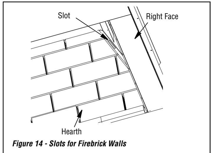
**Figure 14 - Slots for Firebrick Walls**
