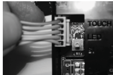
Figure 20 - Connecting end of Touch Pad Cable
