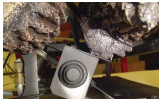
Figure 24A - Installing Front Left Log Side View
