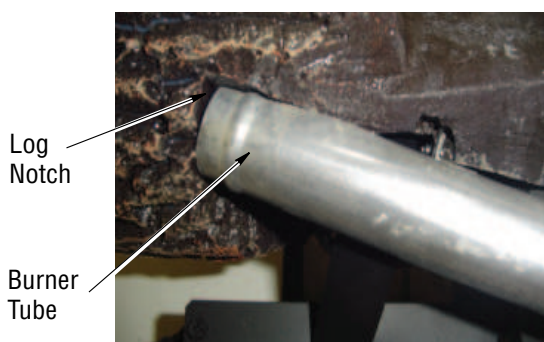
Figure 25A - Installing Back Left Log
