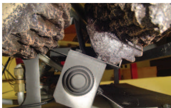
Figure 26A - Installing Front Left Log Side View
