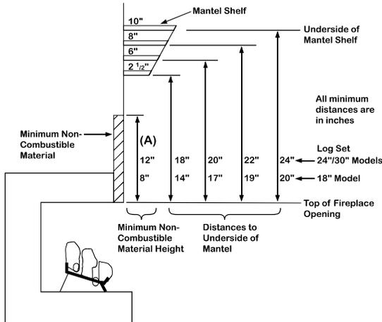
**Figure 6 - Minimum Mantel Clearances Without Using Hood**
