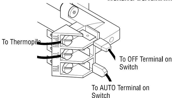
**CAUTION: Label all wires prior to disconnection when servicing controls. Wiring errors can cause improper and dangerous operation. Verify proper operation after servicing.**
