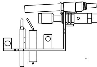
**Figure 68 - Pilot (Natural gas pilot shown)**
