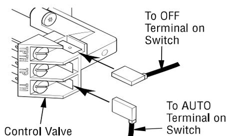
**Figure 18 - Connecting Wires**
