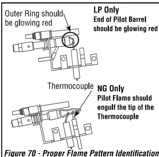
**Figure 70 - Proper Flame Pattern Identification**
