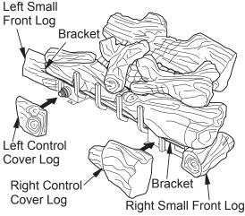
Figure 25 - Installing AndesMtn36 Model Control Cover Logs
