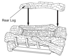
Figure 49 - Installing Rear Log
