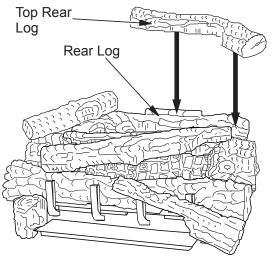
Figure 52 - Installing Top Rear Log
