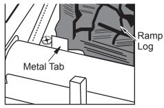
Figure 28 - Installing Log Set
