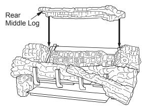
Figure 48 - Installing Rear Middle Log
