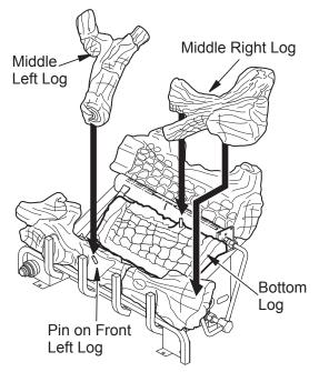
Figure 24 - Installing Log Sets
