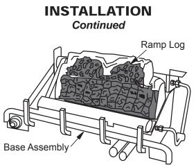
Figure 27 - Installing Log Set
