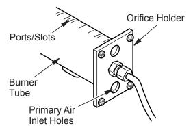
Figure 63 - Orifice Holder On Outlet Burner Tube
