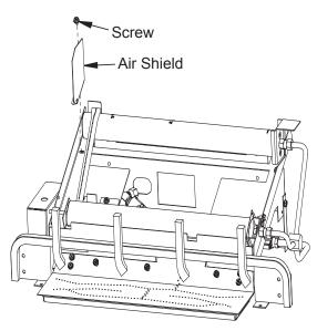
Figure 41 - Removing Air Shield
