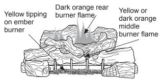
Figure 62 - Incorrect Burner Flame Pattern
