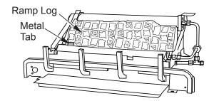
Figure 42 - Installing Fiber Ramp Log
