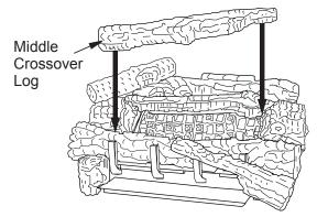
Figure 51 - Installing Middle Crossover Log
