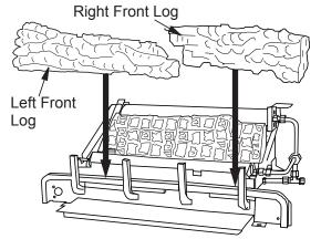
Figure 43 - Installing Left/Right Front Logs
