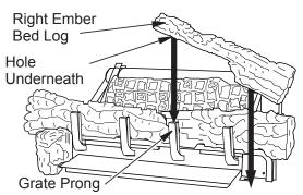
Figure 45 - Installing Right Ember Bed Log
