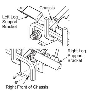
Figure 22-Installing Log Support Brackets
