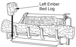
Figure 44 - Installing Left Ember Bed Log
