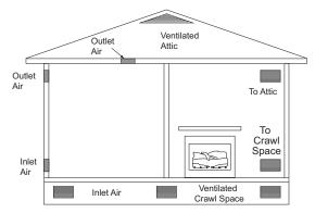
Figure 3 - Ventilation Air from Outdoors
