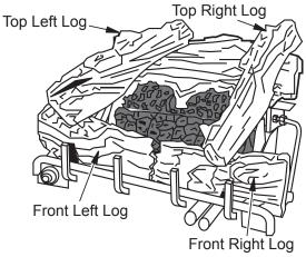
Figure 30 - Installing Logs
