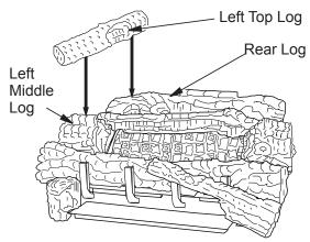
Figure 50 - Installing Left Top Log
