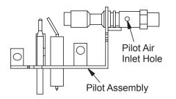
Figure 64 - Pilot Inlet Air Hole (Your pilot may vary from pilot shown)
