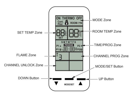
Figure 56 - Touch-Screen LCD and Button Layout
