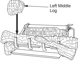
Figure 46 - Installing Left Middle Log
