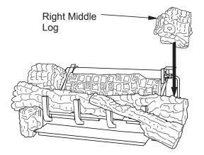
Figure 47 - Installing Right Middle Log
