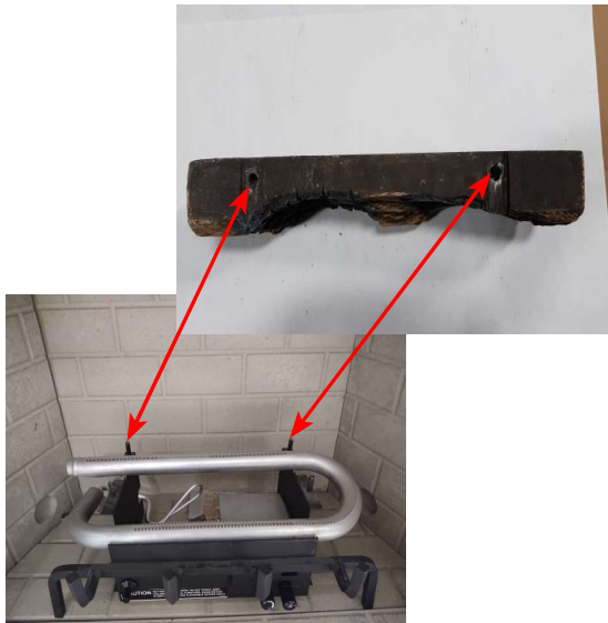
Figure N - Rear Log Placement
