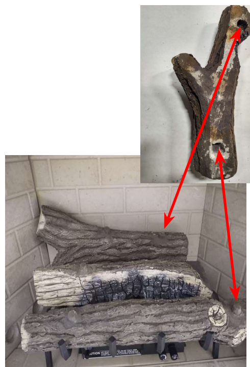
Figure G - Top Right Log Placement
