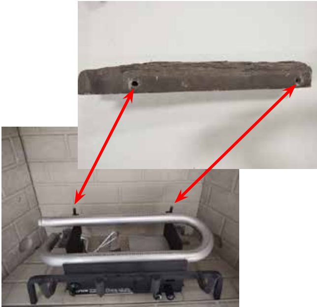
Figure A - Rear Log Placement
