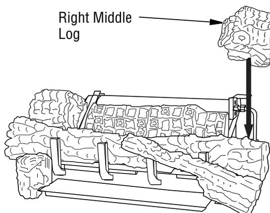
**Figure 29 - Installing Right Middle Log**
