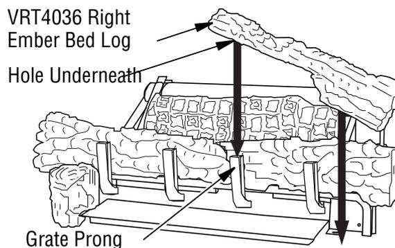
**Figure 27 - Installing Right Ember Bed Log**
