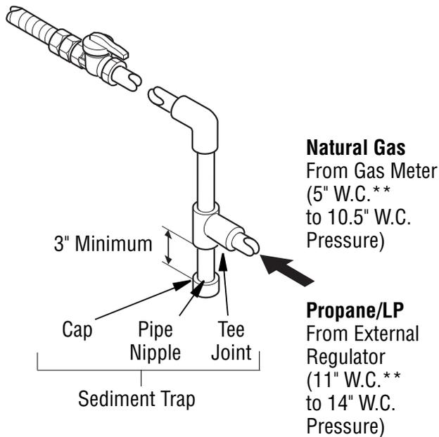
\*\* Minimum inlet pressure for purpose of input adjustment.
