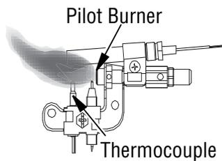
**Figure 42 - Incorrect Pilot Flame Pattern**
