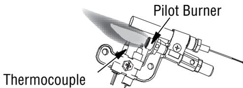
**Figure 41 - Correct Pilot Flame Pattern**
