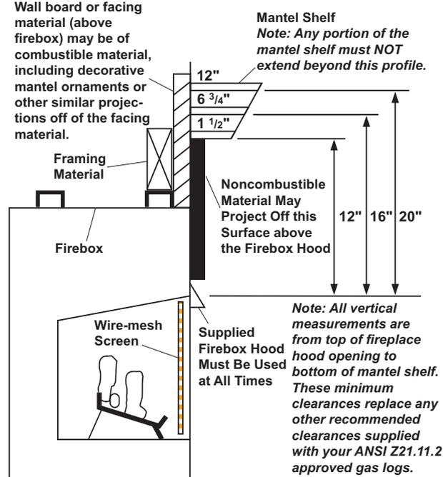
Figure 16 - Minimum Mantel Clearances for Built-In Installation
