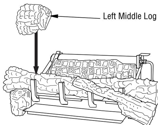
**Figure 28 - Installing Left Middle Log**
