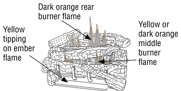
**Figure 44 - Incorrect Burner Flame Pattern**
