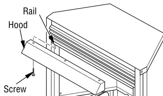
**Figure 5 - Installing Hood**
