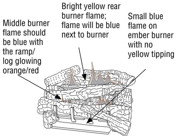
**Figure 43 - Correct Burner Flame Pattern**
