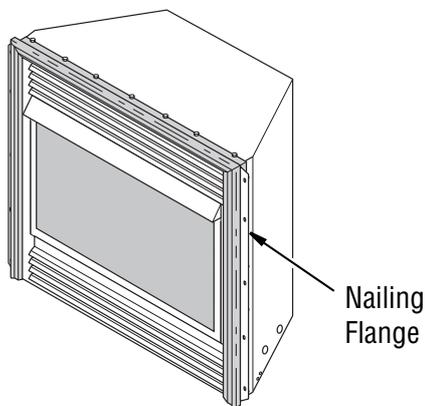
**Figure 11 - Location of Nailing Flange**
