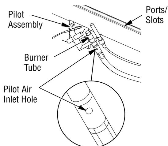
**Figure 46 - Pilot Inlet Air Hole**
