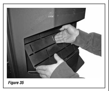
4. Make sure that the brick panel is centered, with equal space on either side of the auger tube. While holding the panel in place, use the drill with a #18 drill bit to drill out the four holes in the back of the firebox, as shown in *Figure 36*.
