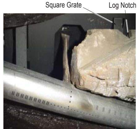
Figure 25B - Installing Charred Log Top Side View
