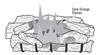
Figure 30 - Incorrect Burner Flame Pattern
