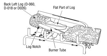
Figure 19 - Installing Back Left Log
