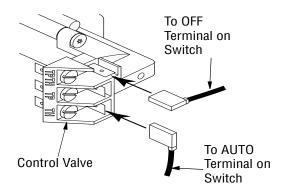
Figure 16 - Connecting Wires
