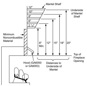
Figure 5 - Minimum Mantel Clearances When Using Hood
