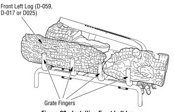
Figure 20 - Installing Front Left Log
