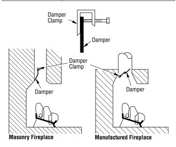
Figure 8 - Attaching Damper Clamp
