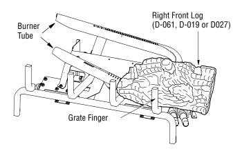
Figure 18 - Installing Right Front Log
