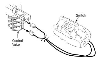
Figure 17- Disconnecting Switch from Control Valve
