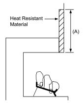
Figure 3 - Heat Resistant Material (Slate, Marble, Tile, etc.)
