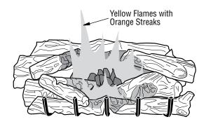
Figure 29 - Correct Burner Flame Pattern
