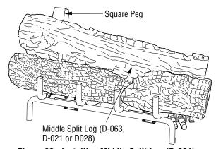
Figure 22 - Installing Middle Split Log (D-021)
