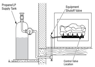
Figure 14- Checking Gas Joints (Propane/LP Only)
