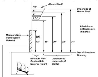
Figure 4 - Minimum Mantel Clearances Without Using Hood
