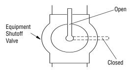
Figure 13 - Equipment Shutoff Valve
