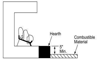
Figure 7 - Minimum Fireplace Clearances Above Combustible Flooring
