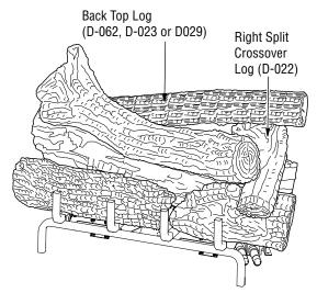
Figure 25 - Installing Back Top Log and Final Assembly
