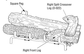
Figure 23 - Installing Right Split Crossover Log
