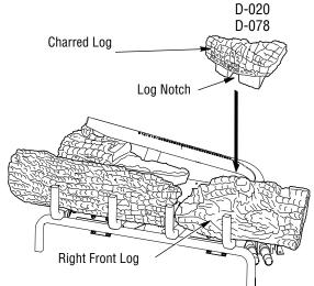
Figure 21 - Installing Charred Log
