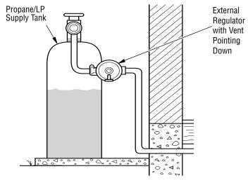
Figure 11 - External Regulator With Vent Pointing Down
