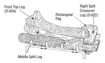
Figure 24 - Installing Front Top Log
