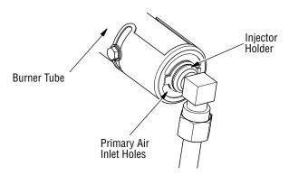
Figure 31 - Injector Holder On Outlet Burner Tube
