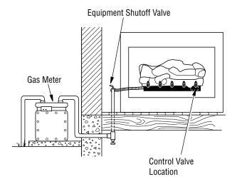
Figure 15 - Checking Gas Joints (Natural Gas Only)
