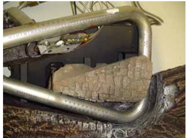
Figure 20A - Installing Charred Log Top View
