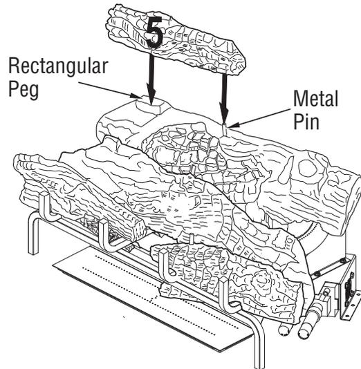
**Figure 26 - Installing Log # 5**
