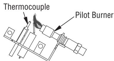
**Figure 55 - Incorrect Pilot Flame Pattern (Your pilot may vary from pilots shown)**
