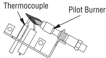
**Figure 54 - Correct Pilot Flame Pattern (Your pilot may vary from pilots shown)**
