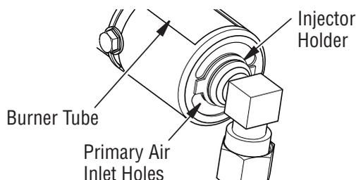
**Figure 56 - Injector Holder On Outlet Burner Tube**
