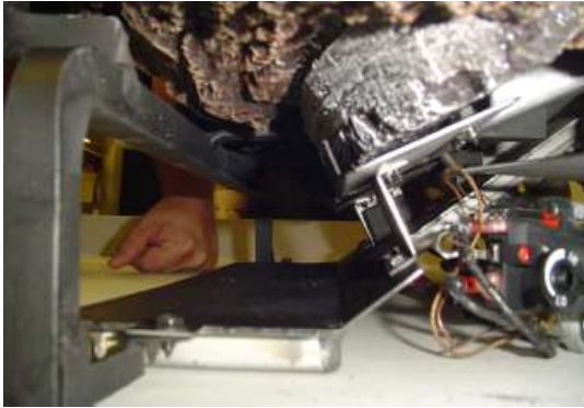
Figure 22C - Installing Right Front Log, Side View
