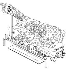
Figure 40 - Installing Log # 3
