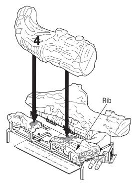
Figure 24 - Installing Log #4
