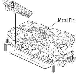
Figure 31 - Installing Log # 3
