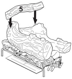
Figure 25 - Installing Log #5
