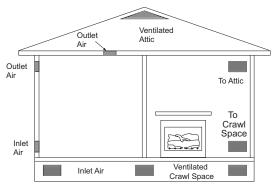
Figure 3 - Ventilation Air from Outdoors
