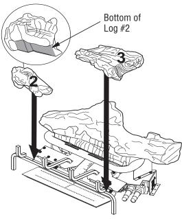
Figure 23 - Installing Logs #2 and #3
