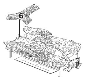
Figure 34 - Installing Log # 6
