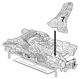
Figure 35 - Installing Log # 7
