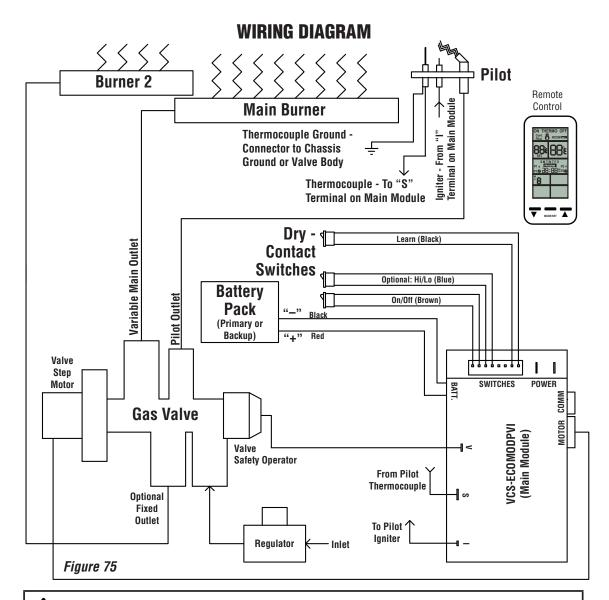
**CAUTION:** Label all wires prior to disconnection when servicing controls. Wiring errors can cause improper and dangerous operation. Verify proper operation after servicing.
