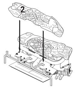
Figure 30 - Installing Log # 2
