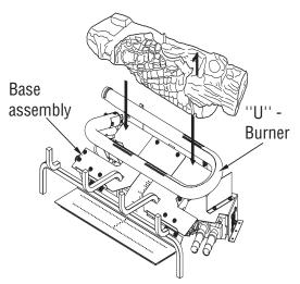
Figure 38 - Installing Log # 1
