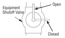
Figure 14 - Equipment Shutoff Valve
