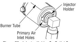
Figure 73 - Injector Holder On Outlet Burner Tube
