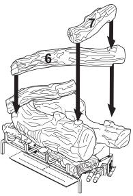
Figure 26 - Installing Logs #6 and #7
