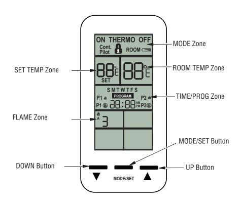
Figure 68 - Touch-Screen LCD and Button Layout
