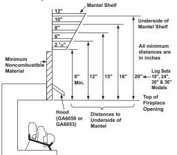
Figure 7 - Minimum Mantel Clearances When Using Hood
