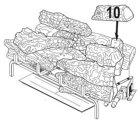
Figure 47 - Installing Log # 10
