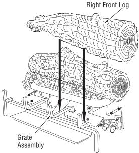
Figure 52 - Installing Right Front Log
