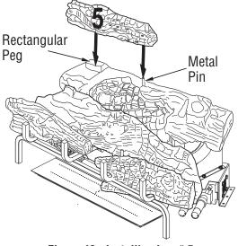
Figure 42 - Installing Log # 5
