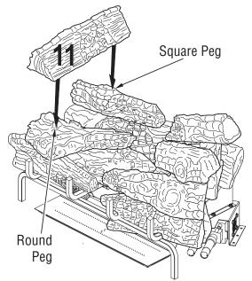
Figure 48 - Installing Log # 11
