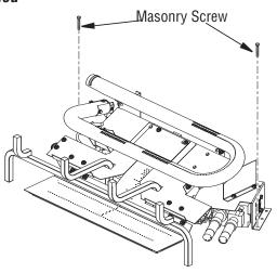
Figure 11 - Attaching Base to Fireplace Floor
