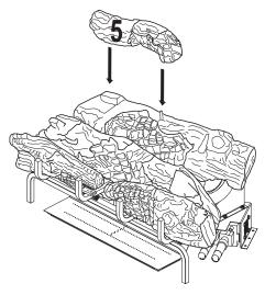
Figure 33 - Installing Log # 5
