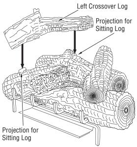
Figure 55 - Installing Left Crossover Log
