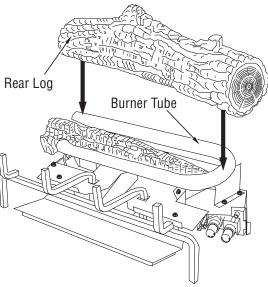
Figure 51 - Installing Rear Log
