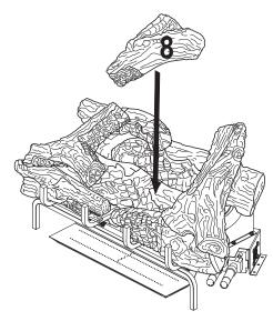
Figure 36 - Installing Log # 8
