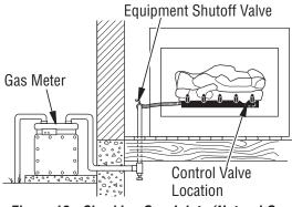
Figure 16 - Checking Gas Joints (Natural Gas Only)
