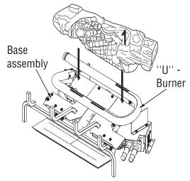
Figure 29 - Installing Log # 1
