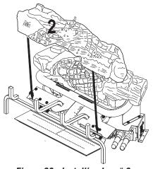
Figure 39 - Installing Log # 2
