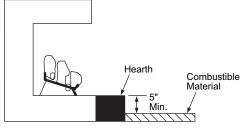
Figure 9 - Minimum Fireplace Clearances Above Combustible Flooring
