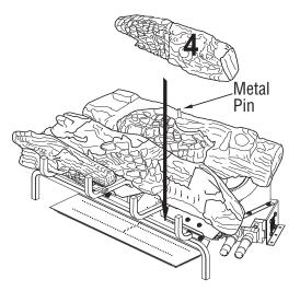
Figure 32 - Installing Log # 4
