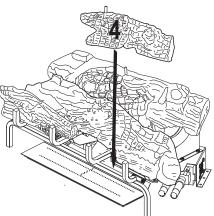
Figure 41 - Installing Log # 4
