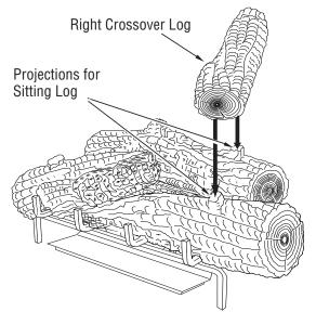
Figure 54 - Installing Right Crossover Log
