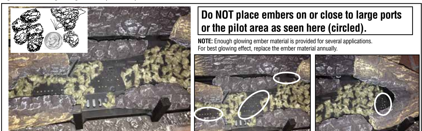
Figure 49 - Place glowing embers (rockwool)
