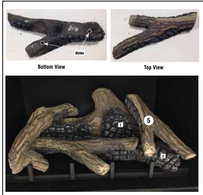
Figure 45 - Install right twig log (5)
