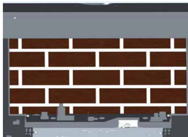
Figure 39A - Install Rear Fiber Panel
