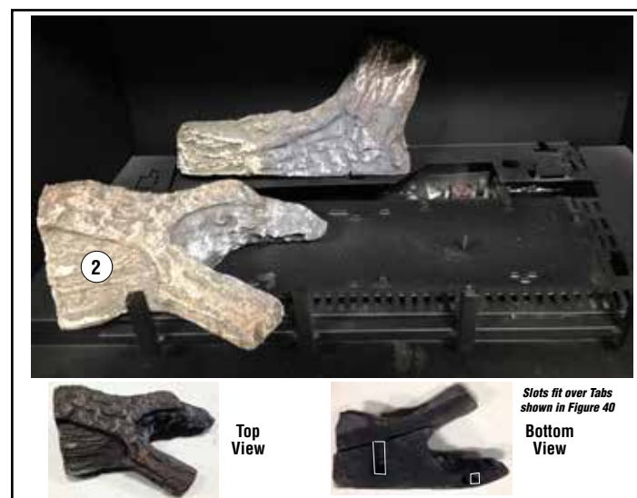
Figure 42 - Place left front bottom log (2)
