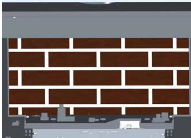
Figure 39A - Install Rear Fiber Panel
