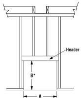
\* Increase Framing Height By 3/4" When Using Optional Drain Pan
