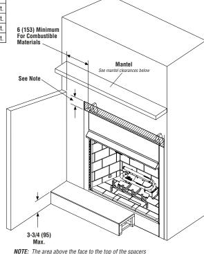
NOTE: The area above the face to the top of the spacers must be non-combustible materials.
