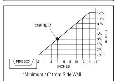
Figure 4 - Minimum Clearance for Combustible to Wall
