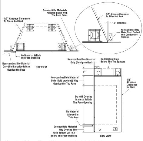
Figure 5 - Minimum Mantel Clearances for Built-In Installation
