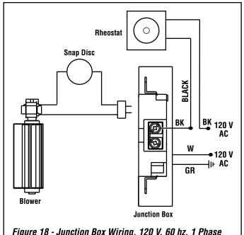
Figure 18 - Junction Box Wiring, 120 V, 60 hz, 1 Phase
