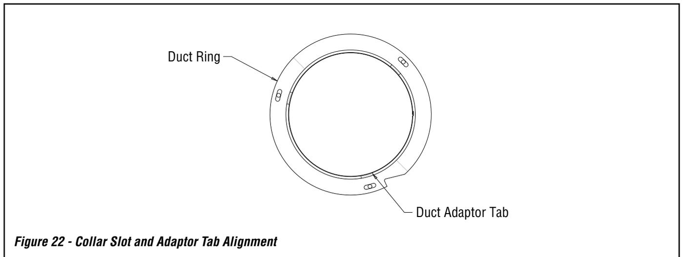
**Figure 22 - Collar Slot and Adaptor Tab Alignment**
