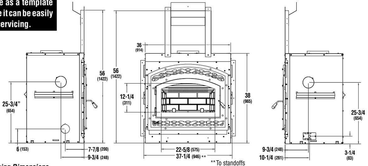
**Figure 11 - Framing Dimensions**
