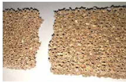
Combustor Problem - Broken Combustor
