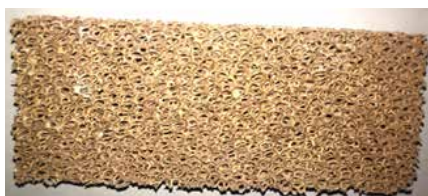
Combustor Problem - Cracked Combustor
