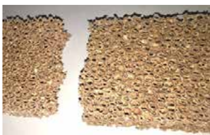
Combustor Problem - Broken Combustor
