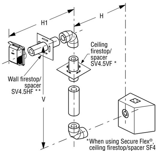
\*When using Secure Flex®, use ceiling firestop/spacer SF4.5VF.
