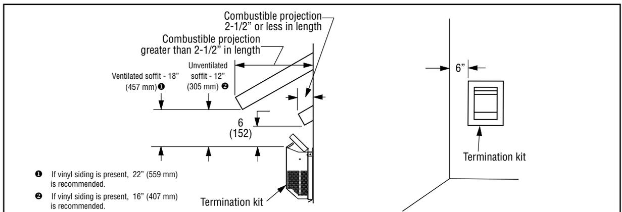
**Table 7 - Horizontal vent termination clearances for buildings with combustible and noncombustible exteriors**
