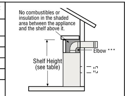
\* Includes 3" clearance to combustibles (required above vent components)
