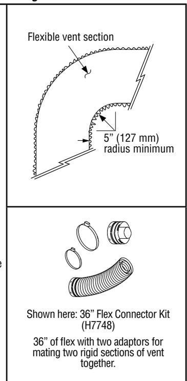
1. Install the Inner Flex Pipe.
