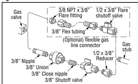
These fireplaces are equipped with a gas flex line for use (where permitted) in connecting the unit to the gas line. A gas flex line is provided to aid in attaching the direct-vent fireplace to the gas supply. The gas flex line can only be used where local codes permit. The flex line is rated for both natural and propane gas. A manual shut off valve is also provided with the flex line.
