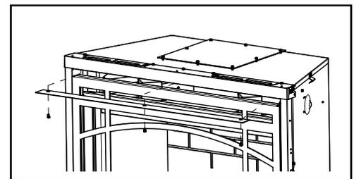
**22. Installation / Re-installation of the required facade / barrier**
