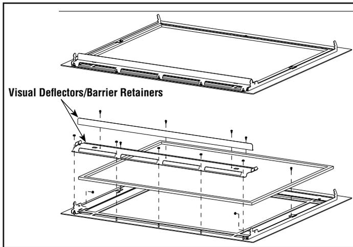
Figure 36D - Bend Retaining TAB UP
