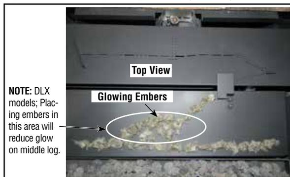
**Figure 42B - Install glowing embers (AltairDLX-C)**
