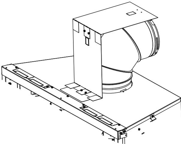
**STEP 5.** Fold down tab to support rear of shield.
