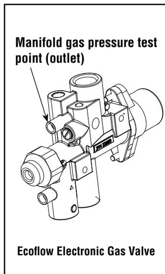
**Figure 1B - Appliances With 1/8" NPT plug (inlet test point)**
