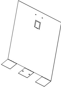
**STEP 3.** Attach the two (2) shields, as shown, with screws.
