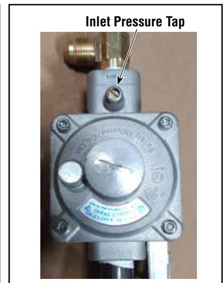
Propane tanks are at pressures that will cause damage to valve components. Verify that the tanks have step down regulators to reduce the pressure to safe levels.
