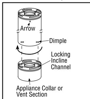
**Figure 15B - Connected vent components**
