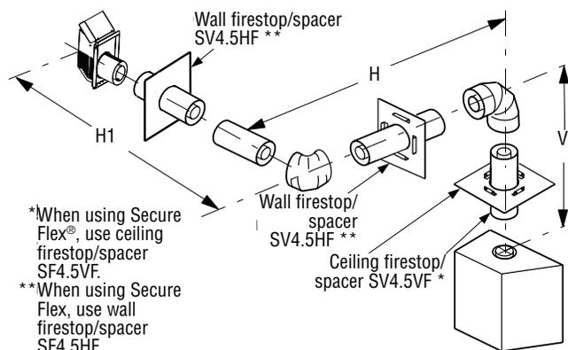
\*When using Secure Flex®, use ceiling firestop/spacer SF4.5VF.
