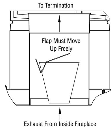
**Figure 14B - Vent restrictor installation, Rear vent**
