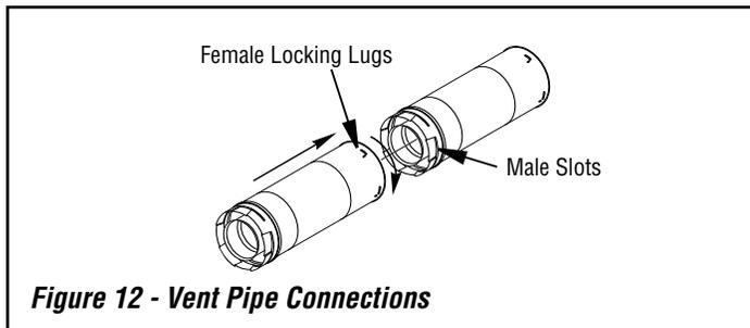
**Figure 12 - Vent Pipe Connections**
