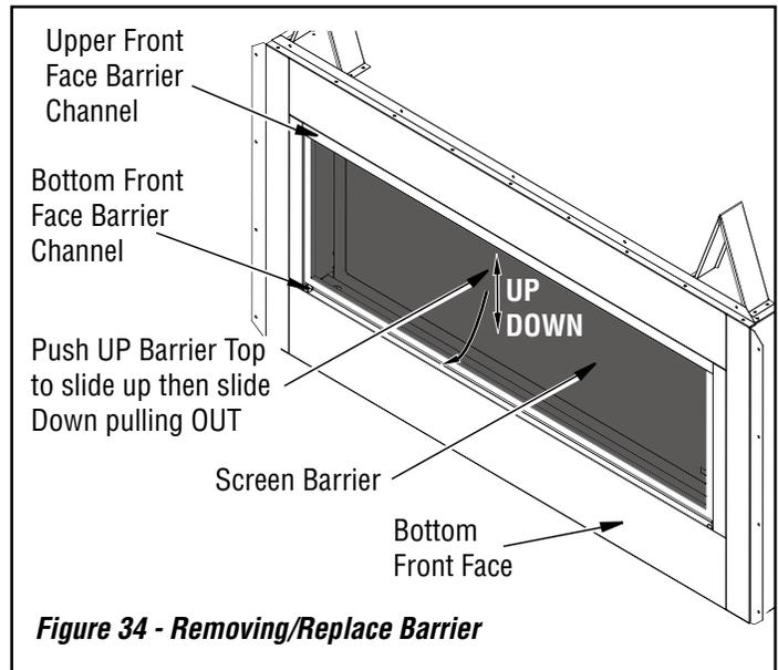
**Figure 34 - Removing/Replace Barrier**
