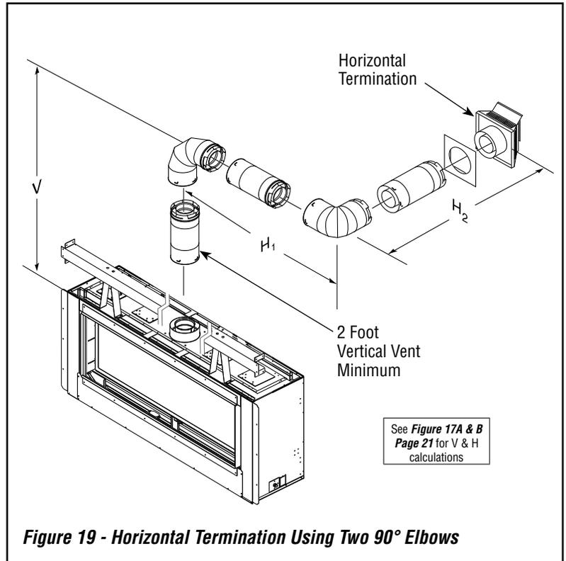
**Figure 19 - Horizontal Termination Using Two 90° Elbows**
