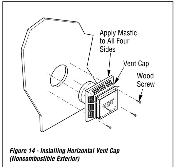
**Figure 14 - Installing Horizontal Vent Cap (Noncombustible Exterior)**
