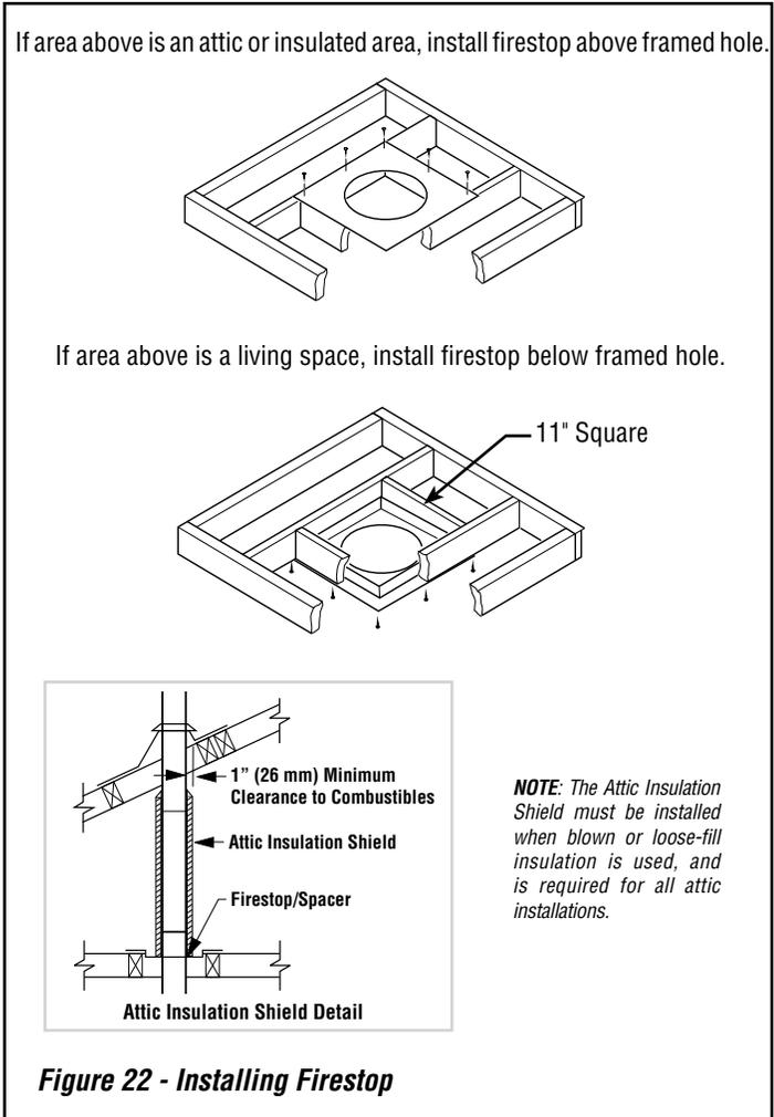
3. Cut a hole in the roof using locating hole as a center point. (Cover any exposed open vent pipes before cutting hole in roof.) The 11"x 11" hole must be measured on the horizontal; actual length may be larger depending on pitch of roof. There must be a 1" clearance from vent pipe to combustible materials. Frame opening as shown in **Figure 22**.
