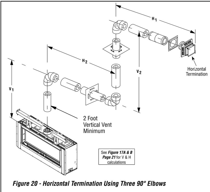
**Figure 20 - Horizontal Termination Using Three 90° Elbows**
