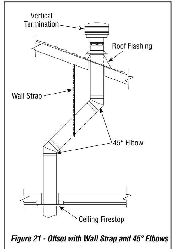
**Figure 21 - Offset with Wall Strap and 45° Elbows**
