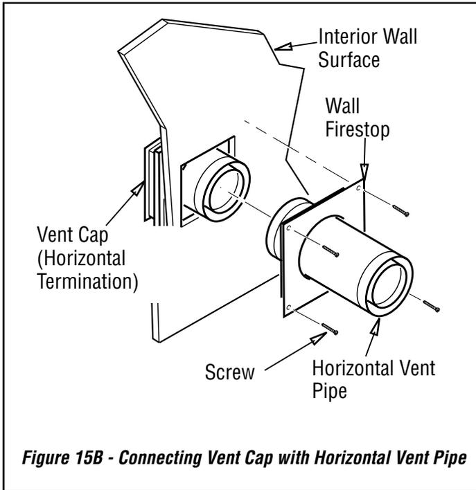
**Figure 15B - Connecting Vent Cap with Horizontal Vent Pipe**
