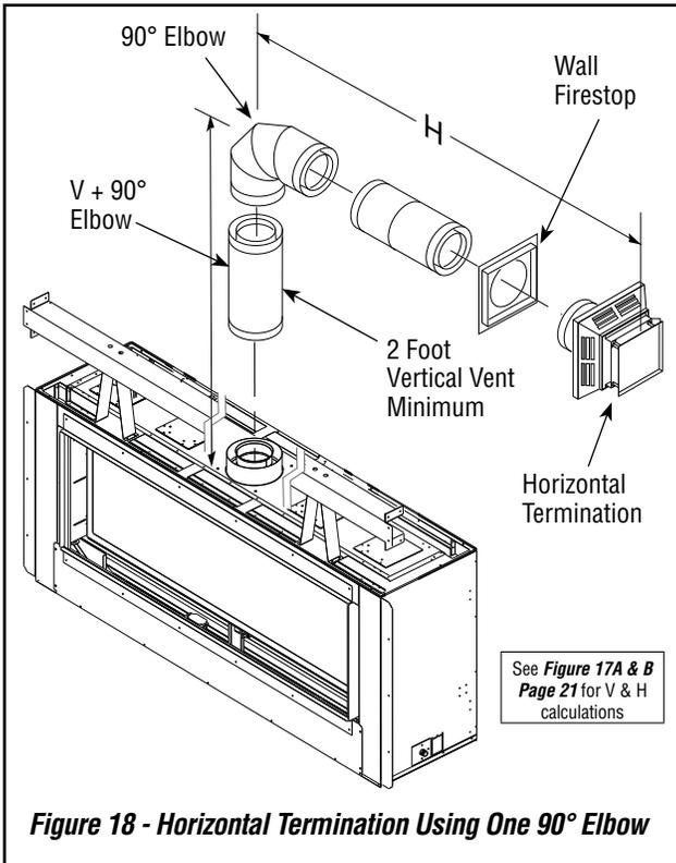
**Figure 18 - Horizontal Termination Using One 90° Elbow**
