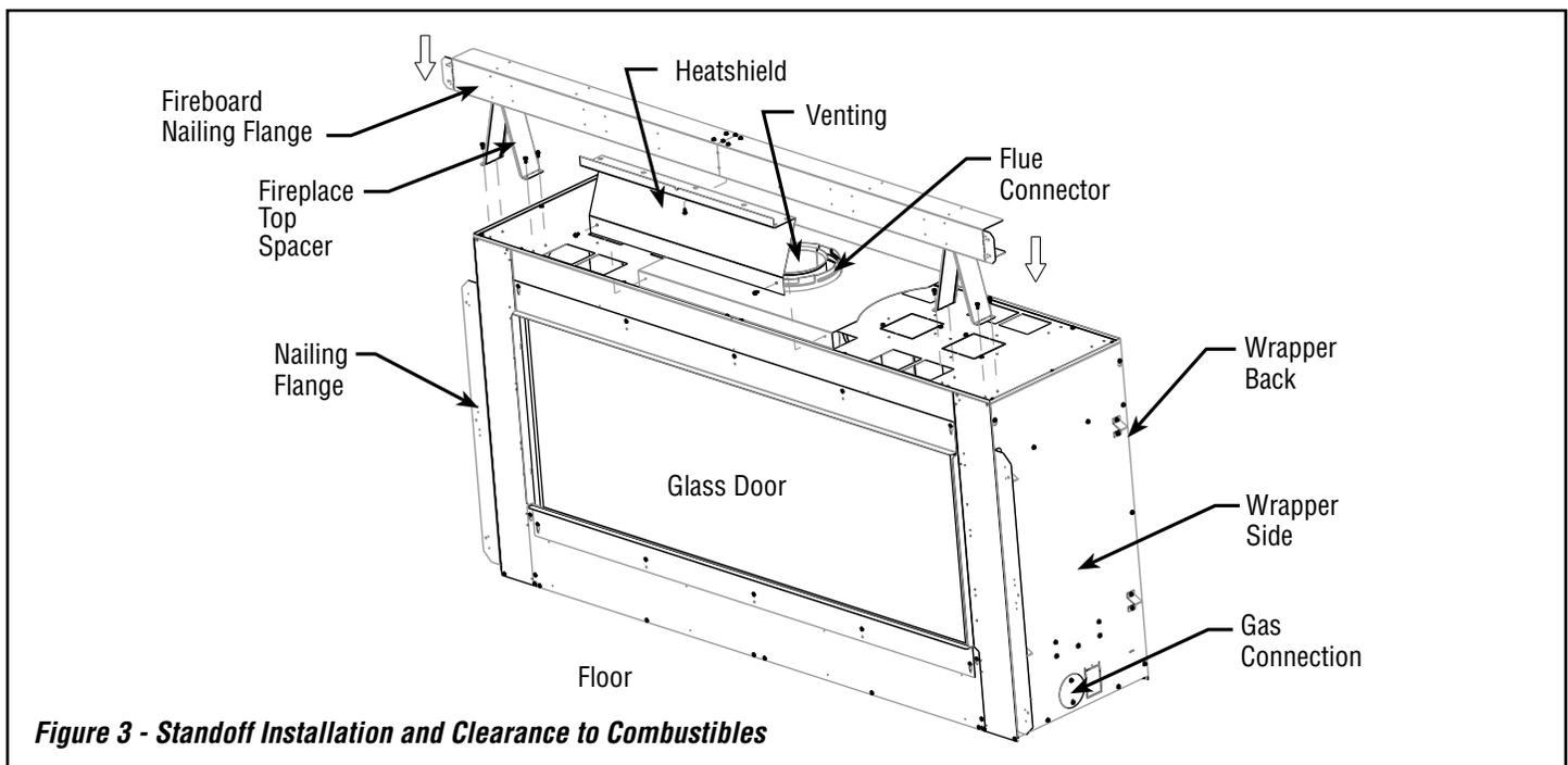
**Figure 3 - Standoff Installation and Clearance to Combustibles**
