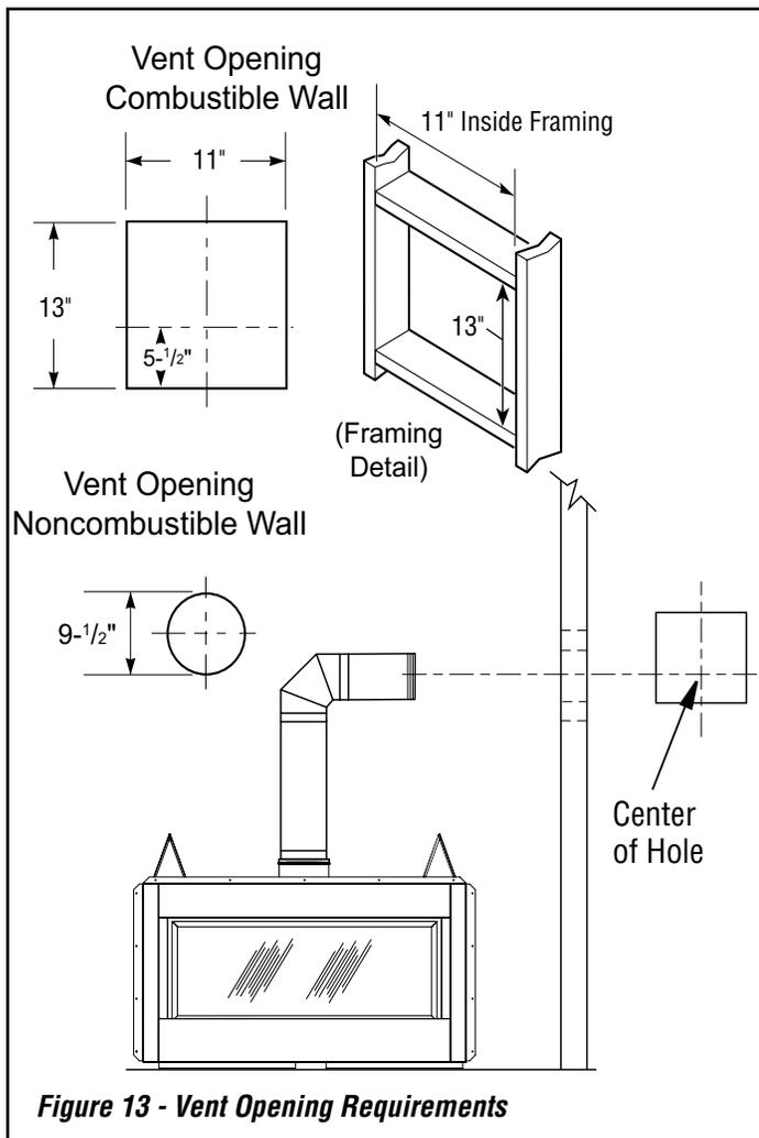
**Figure 13 - Vent Opening Requirements**
