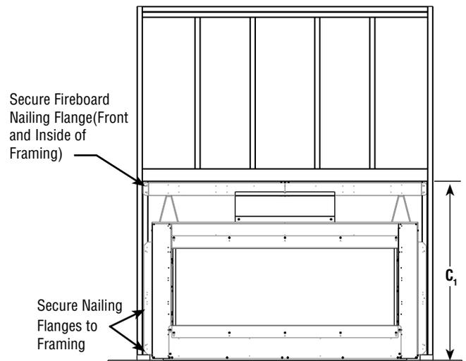
**Figure 4 - Framing Flush Wall (Standard Installation)**
