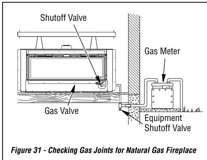
**Figure 31 - Checking Gas Joints for Natural Gas Fireplace**
