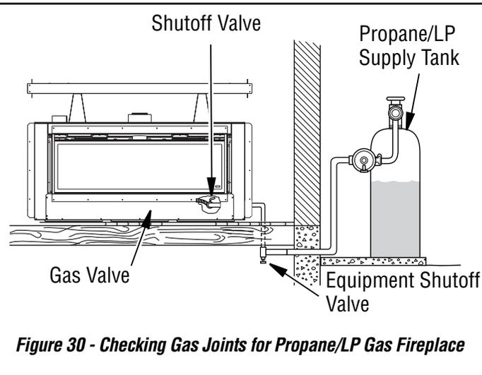
**Figure 30 - Checking Gas Joints for Propane/LP Gas Fireplace**
