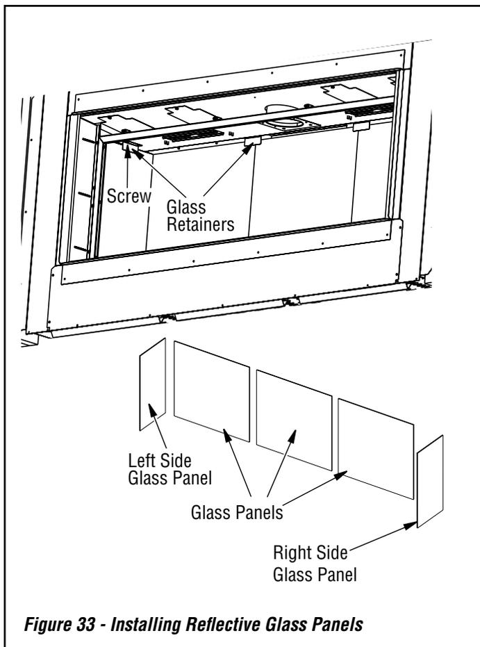
**Figure 33 - Installing Reflective Glass Panels**
