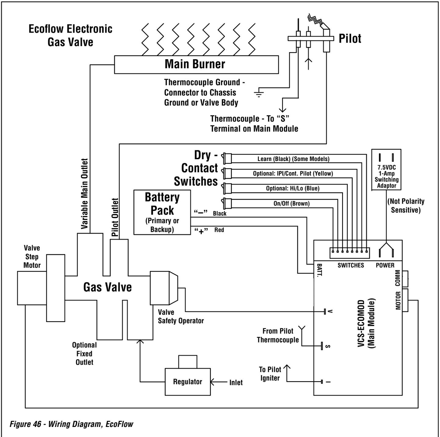
Figure 46 - Wiring Diagram, EcoFlow
