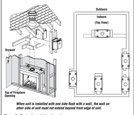
Figure 2 - Typical Installation/Locations
