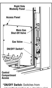
\*ON/OFF Switch: Switches from intermittent ignition to a standing pilot (a standing pilot stays lit when fireplace is OFF).
