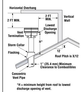
Vent/air intake termination clearances above the high side of an angled roof are listed in the table below.
