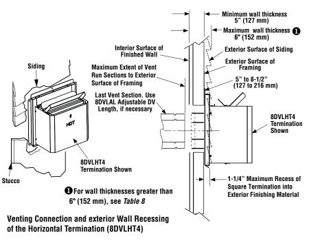
Figure 31—Wall Thickness and Horizontal Termination Requirements
