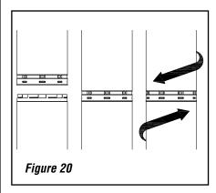
Joint Connection - 8" DV LOCK Direct Vent components are engineered for easy twist lock assembly. Eight indentations are located on the female end of pipe and fittings to slide straight into the male end of the adjacent pipe or fitting, by orientating the eight indentations so they match and slide into the eight entry slots on the male ends.
