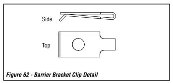
13. Install the barrier bracket clips for additional screw thread.
