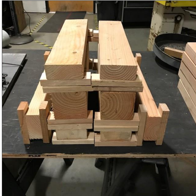
Typical Test Fuel Load Configuration
