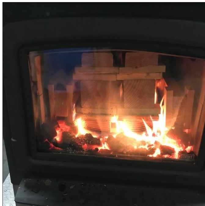
Typical Test Fuel Loaded in Test Stove
