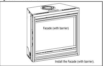
NOTICE: All Aries-E series fireplaces <u>require a facade</u> <u>kit (Vista Facade is included with purchase)</u>, <u>which includes</u> a barrier to reduce the risk of burns from the hot viewing glass. This facade kit must be installed prior to operation.
