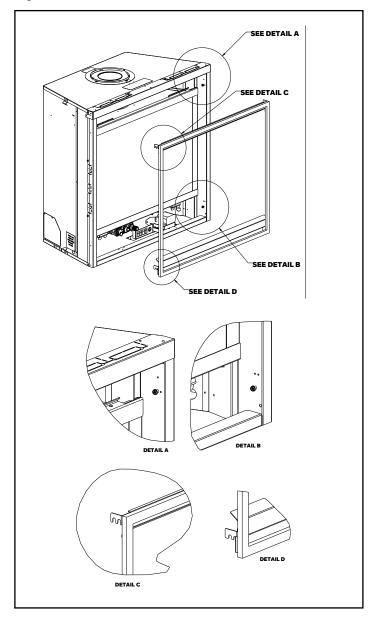
Figure 36B - Facade Installation
