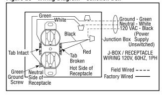
**NOTE:** This outlet as shown must be wired directly to the AC breaker box so the bottom receptacle is not switched. This also is the configuration needed for the optional FBK-250 blower.
