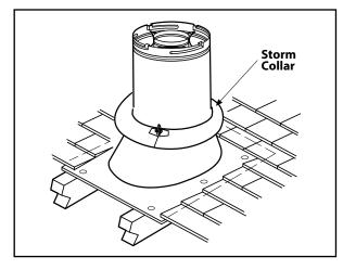
Figure 22 - Installing the Vertical Termination
