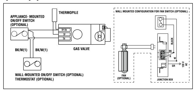
Figure 29 - Wiring Diagram—Junction Box
