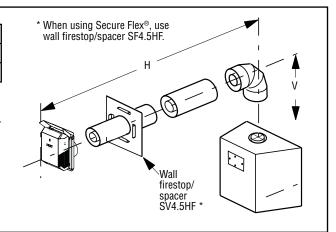
Table 23 - Top Vent—One 90° Elbow, Elbow Connection NOT at Fireplace
