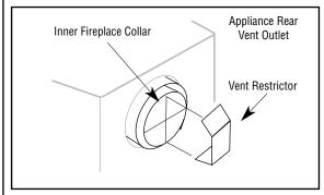
Figure 13C - Vent restrictor assembly
