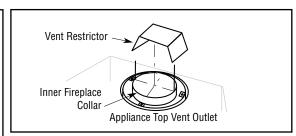
Figure 13B - Vent restrictor installation, Rear vent
