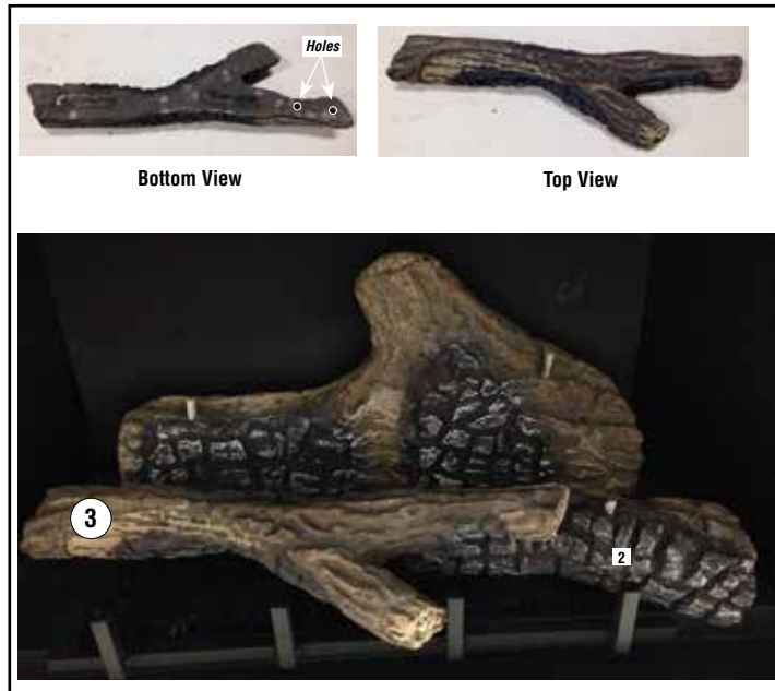
Figure 44 - Install left bottom log (3)
