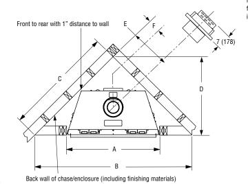
NOTE: When in top vent mode - No combustible material shall be allowed to contact the rear flue cap/cover.
