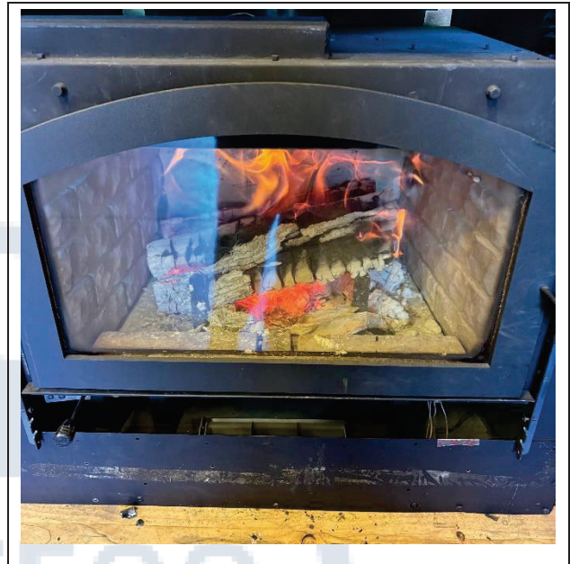
L2 Residual Fuel Loaded
