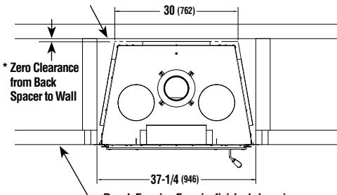
\* Zero Clearance from Back Spacer to Wall
