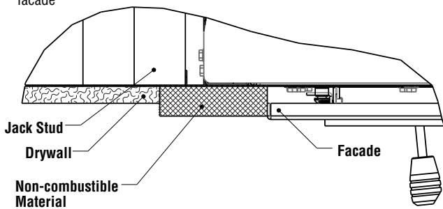
4. Proud install with non-combustible material flush with facade.
