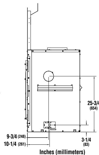
**Figure 11 - Framing Dimensions**
