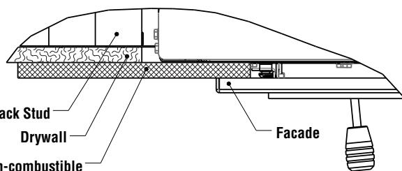
2. Standard flush install with non-combustible material flush with facade
