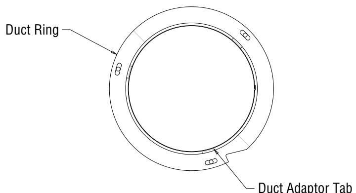
Figure 22 - Collar Slot and Adaptor Tab Alignment
