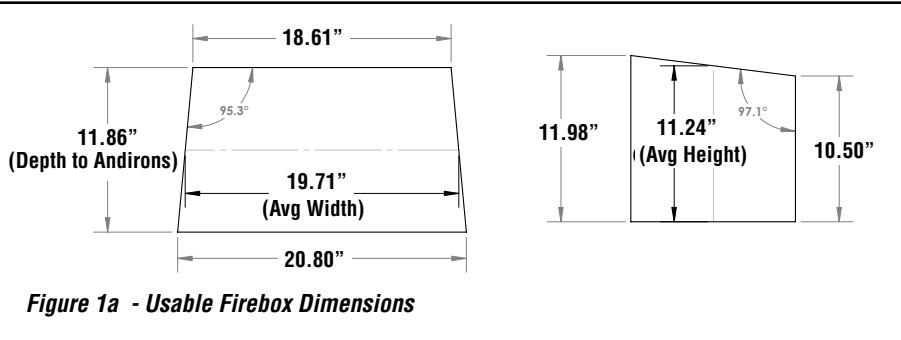
Figure 1a - Usable Firebox Dimensions
