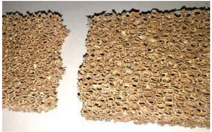
Combustor Problem - Broken Combustor
